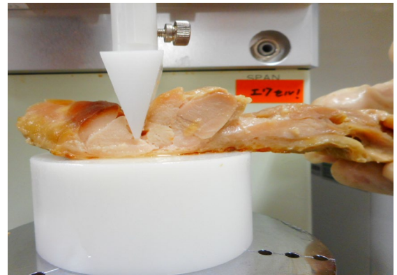
The measurement of the break stress with the creep meter
