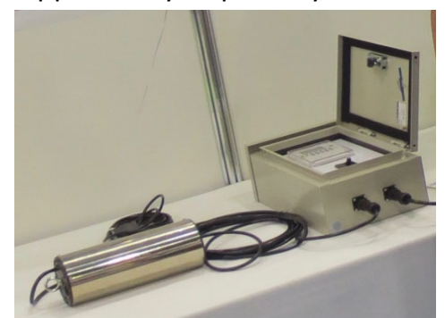
AC electrolysis machine
